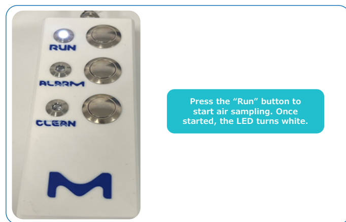
Figure 18: Control box - White LED indicates air sampling has started
