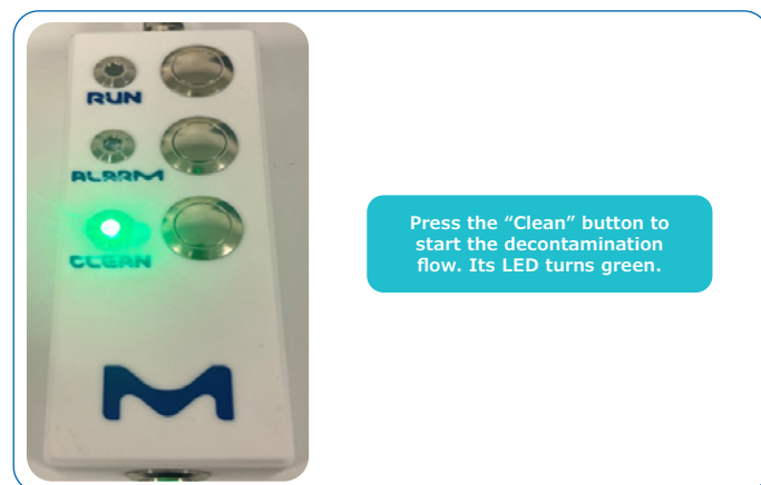
Figure 19: Control box - Clean (decontamination) in progress
