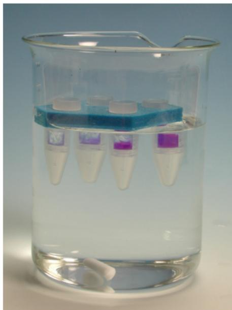
Figure 1: Dialysis with Mini Pur-A-Lyzer.
