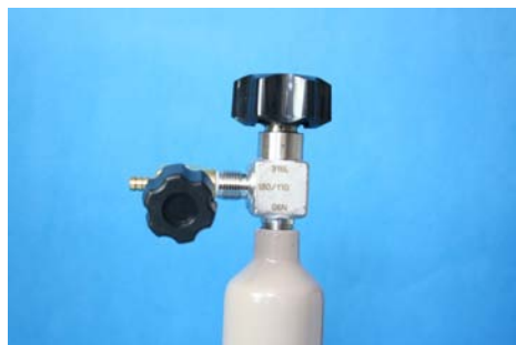
Control valve designated for extremely corrosive gases to meter the flow of gas. WARNING: Gas-control valves do not control pressure in a closed system. Regulator or relief valves should be used to prevent the buildup of unsafe pressures that could lead to explosion.
