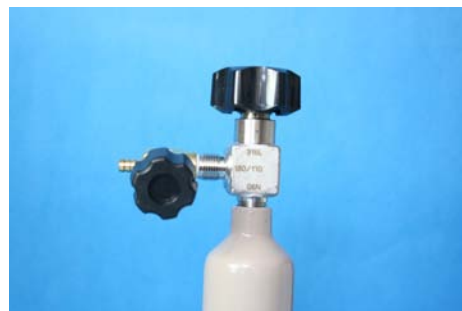
Control valve designated for non-corrosive gases to meter the flow of gas. WARNING: Gas-control valves do not control pressure in a closed system. Regulator or relief valves should be used to prevent the buildup of unsafe pressures that could lead to explosion.
